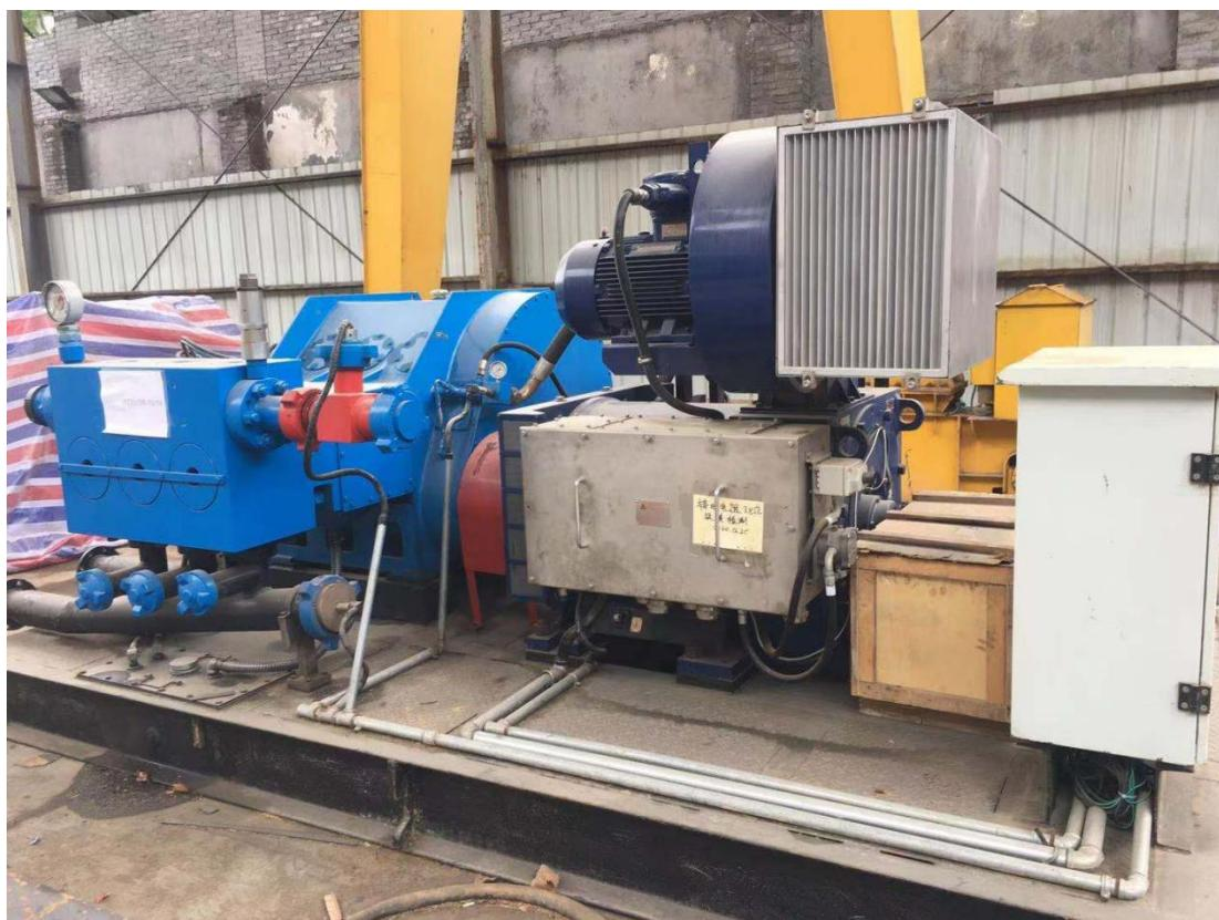
Application: Intermittent work in the oil and gas wells, such fracturing, cementing and completion.
