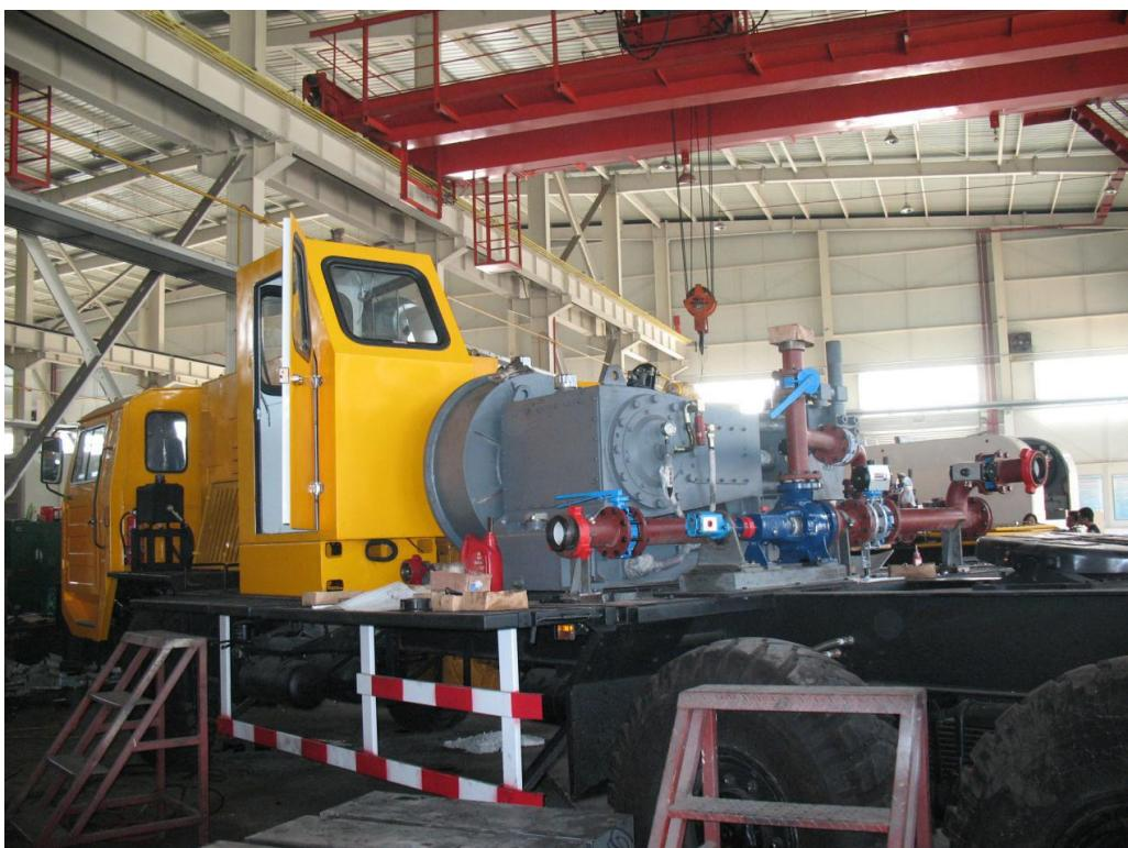
NB Series horizontal triplex plunger Fracture Pumps are specially used to deliver various viscous and non-viscous hydraulic fluids such as fresh water and mud as the trenchless large-tonnage horizontal directional drilling device. It was designed based on the existing mature mud pumps to meet with the wild trenchless directional drilling equipment market demands.
